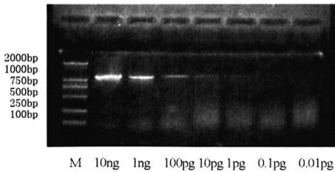
**Figure 1.** The sensitivity of a universal PCR assay. Serial dilutions of *E. coli* DNA and cells were amplified with primers Pba1 and Pba2 and run on an agarose gel. Molecular marker sizes are given on the left in base pairs.
