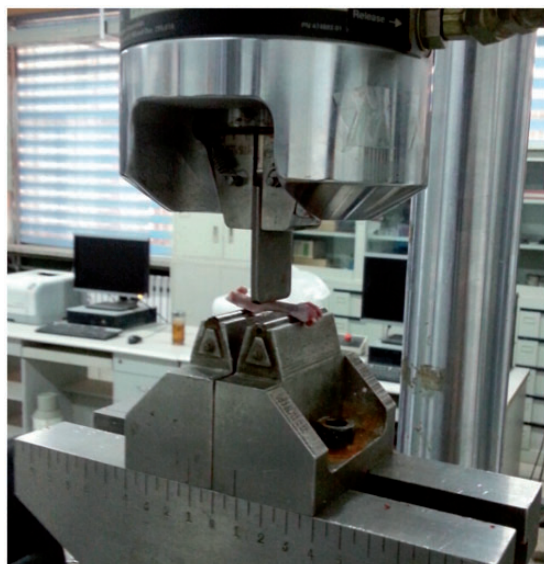
Figure 1 Three-point bending test using a materials testing system. The femurs were immobilized on a fixed support with two loading points with a 20-mm interval distance. The upper loading points were located at the midpoint between the two lower loading points. Then, the load was applied at a constant speed of 2 mm/min until bone fracture occurred. (A color version of this figure is available in the online journal.)
