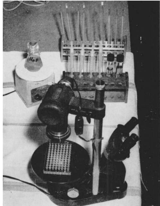
FIG. 1. Microtitration apparatus for tissue culture techniques. Foreground: Inverted microscope with microplate on the microscope stage. Background: Cell suspension on a magnetic stirrer; micropipets and loops in racks.
