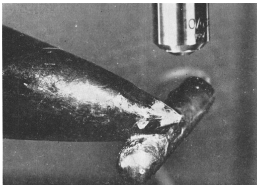
FIG. 1. Photograph of tip of Methacrylate light carrier showing electronic flash tube mounted below.
