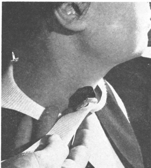
FIG. 1. Special contact microphone cemented to Velcro cuff for placement around the neck.
