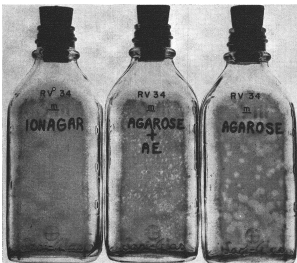
FIG. 2. Effect on m plaque size of agar extract (AE) incorporated into purified agar (agarose).
