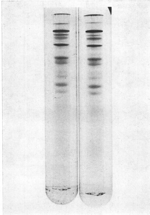
FIG. 2. Photograph of 7.5% polyacrylamide disc gels stained with Coomassie blue after electrophoresis of the denatured proteins of purified herpesvirus type I. The gel on the left is derived from virions produced in Phase II cells and that on the right from virions produced in Phase III cells.
