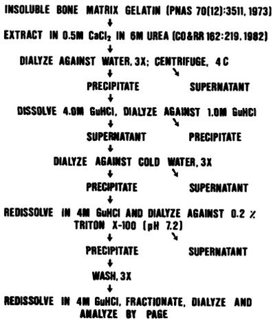
FIG. 1. Flow diagram of a method of chemical extraction of hBMP from cortical bone.
