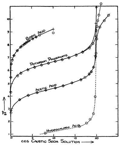
Titration curves obtained with the hydrogen and with the quinhydrone electrodes in the presence of air.
