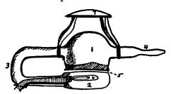
The pressure piece is made of glass. It is composed of an open cup (1) (see drawing) an apposing smooth, slightly convex stage (2), a connecting curved arm (3), and a short glass point (4) by means of which the cup may be connected with the "U" tube. The mouth of the cup is covered by a rubber membrane (5) which, when pressure is made within the cup, bulges against the stage. The rabbit's ear is slipped between the stage and rubber membrane. The stage contains a light
