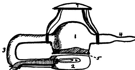
The pressure piece is made of glass. It is composed of an open cup (1) (see drawing) an apposing smooth, slightly convex stage (2), a connecting curved arm (3), and a short glass point (4) by means of which the cup may be connected with the "U" tube. The mouth of the cup is covered by a rubber membrane (5) which, when pressure is made within the cup, bulges against the stage. The rabbit's ear is slipped between the stage and rubber membrane. The stage contains a light
