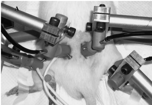
Figure 1. (A) Experimental setup for pressure loading over the trochanter area and tibia area. (B) Schematics of indenter with incorporated probe (diameter = 14 mm).
