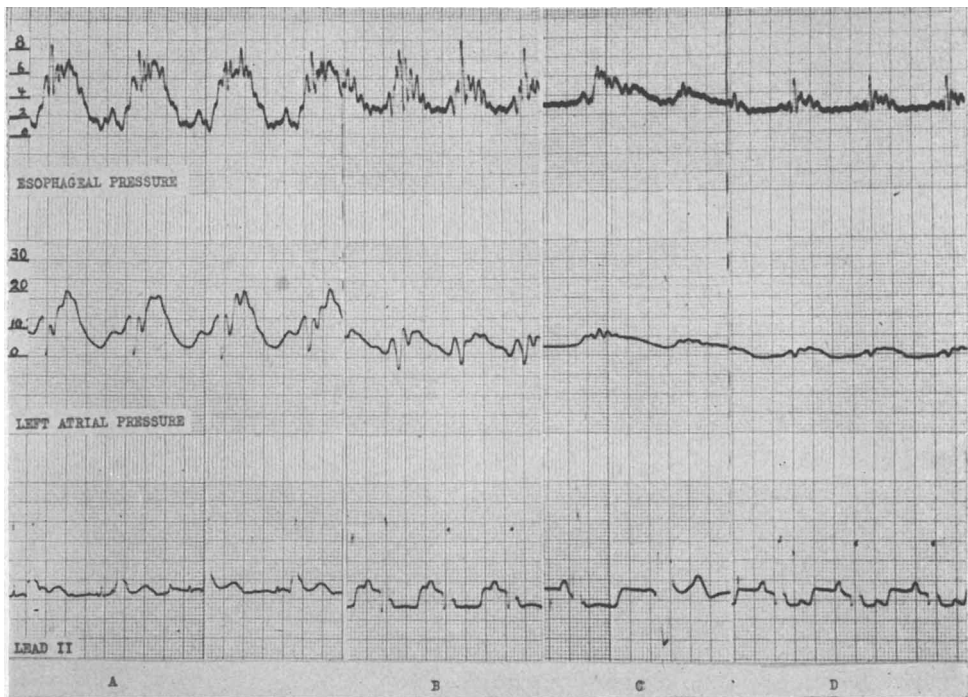
FIG. 2. Tracings A, B, C, and D show successive decline of pulse pressure as the animal was bled to death.
